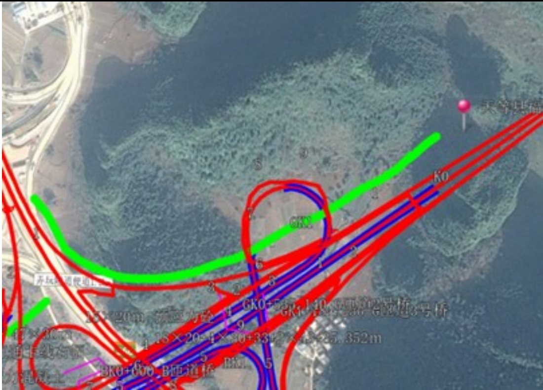
Figure 6.1-15 Location of New Access Road (1.5 km) at G Ramp
