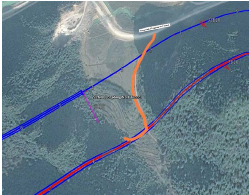
Figure 6.1-23 Location of New Access Road (500m) at Entrance of Longdong No.2 Tunnel
