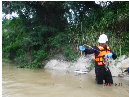
Measure the transparency of surface water with the Sechi Disc.
