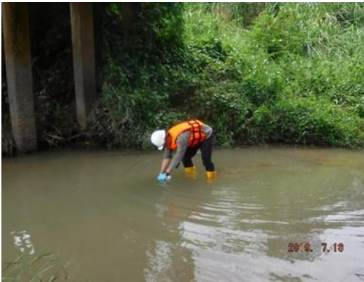
Collect grab sampling in the middle of the canal.
