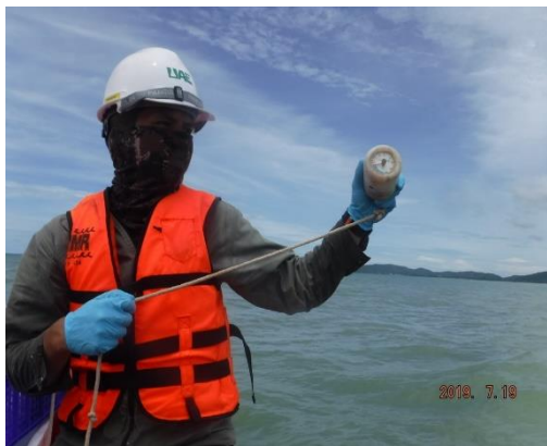
Seawater Transparency Measurement with Secchi Disc
