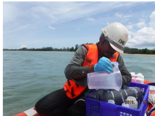
Collect seawater samples in HDPE containers
