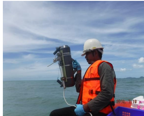
Sampling of marine water with a Teflon Sampler
