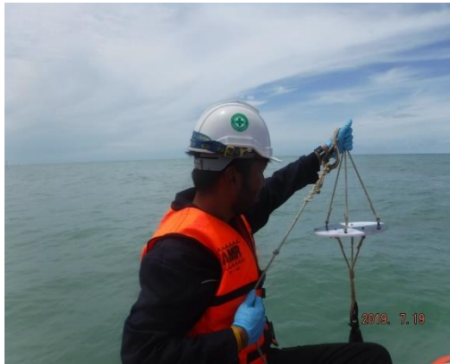
Seawater Transparency Measurement with Secchi Disc
