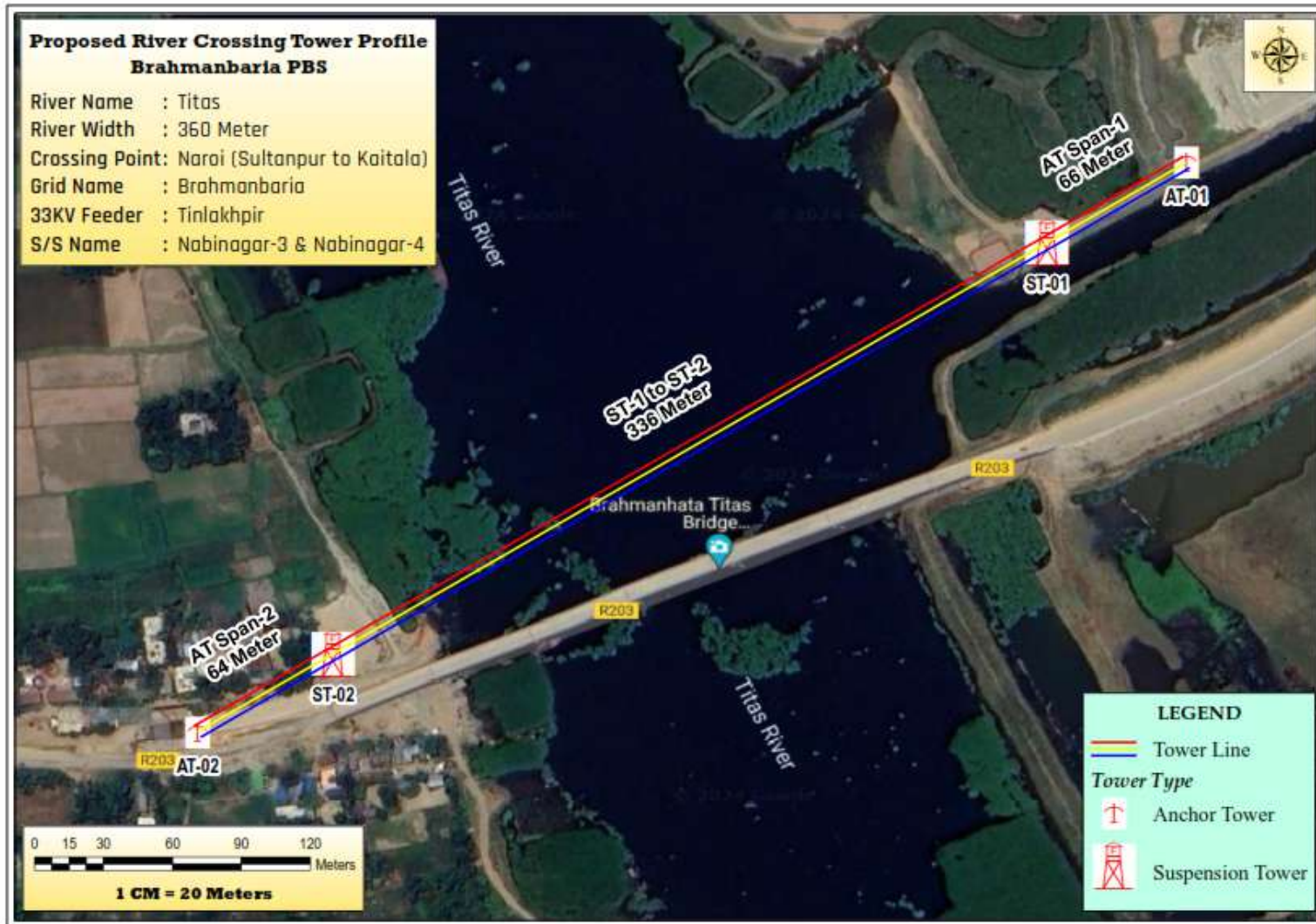
Figure III.9: Proposed Titas River Crossing Tower of Brahmanbaria PBS (Nabinagar-3 & Nabinagar-4)
