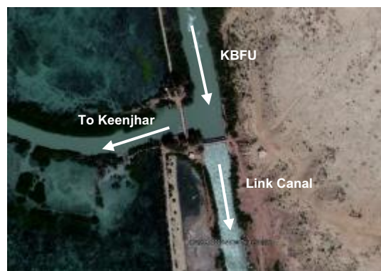
Figure 4-2: Layout of Regulators at -2.4 RD of KBFU
