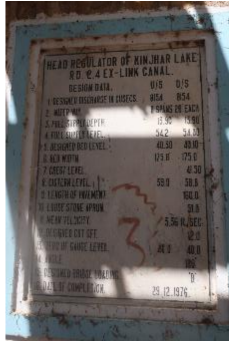
This is the head regulator of Keenjhar Lake at the end of KB Feeder Upper (KBFU) where the water is diverted and controlled to feed Keenjhar Lake, which is built in 1976. The design discharge of the regulator is 8154 cusecs (0.016 MAF per day).
