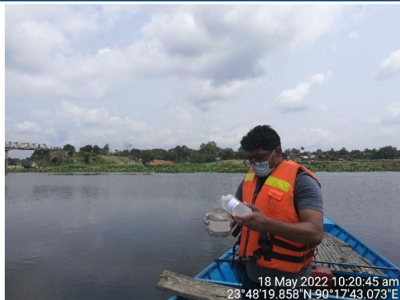
Sample storing and adding 10% buffered formalin in a sample jar
