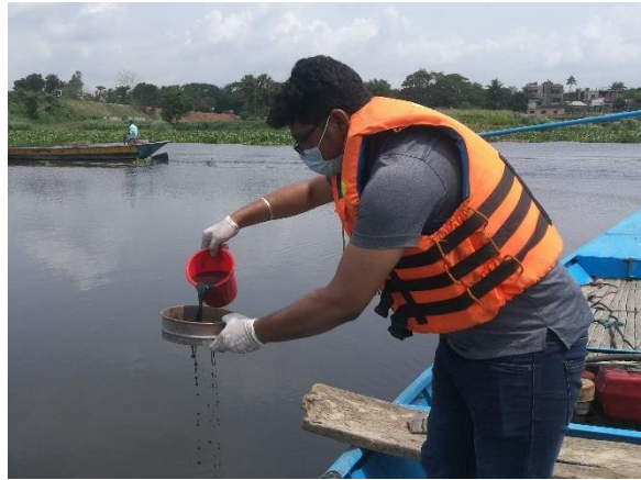
Sample Sieving by 0.5 mm mesh-sized hand sieve
