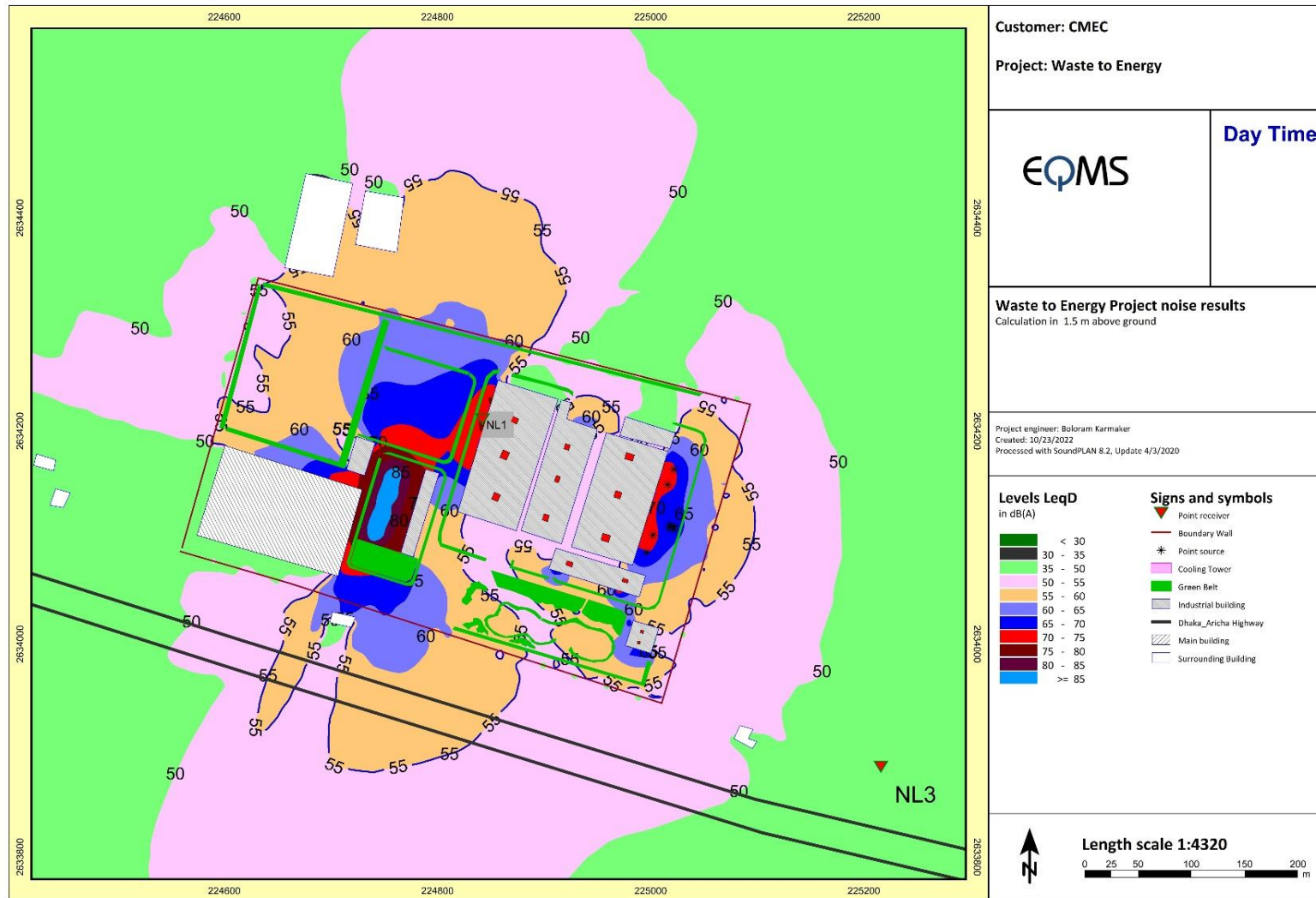
Figure 6-15: Noise contour map for WTE Power Plant North Dhaka Private Limited Waste to Energy Power Plant during the day (Leq day)
