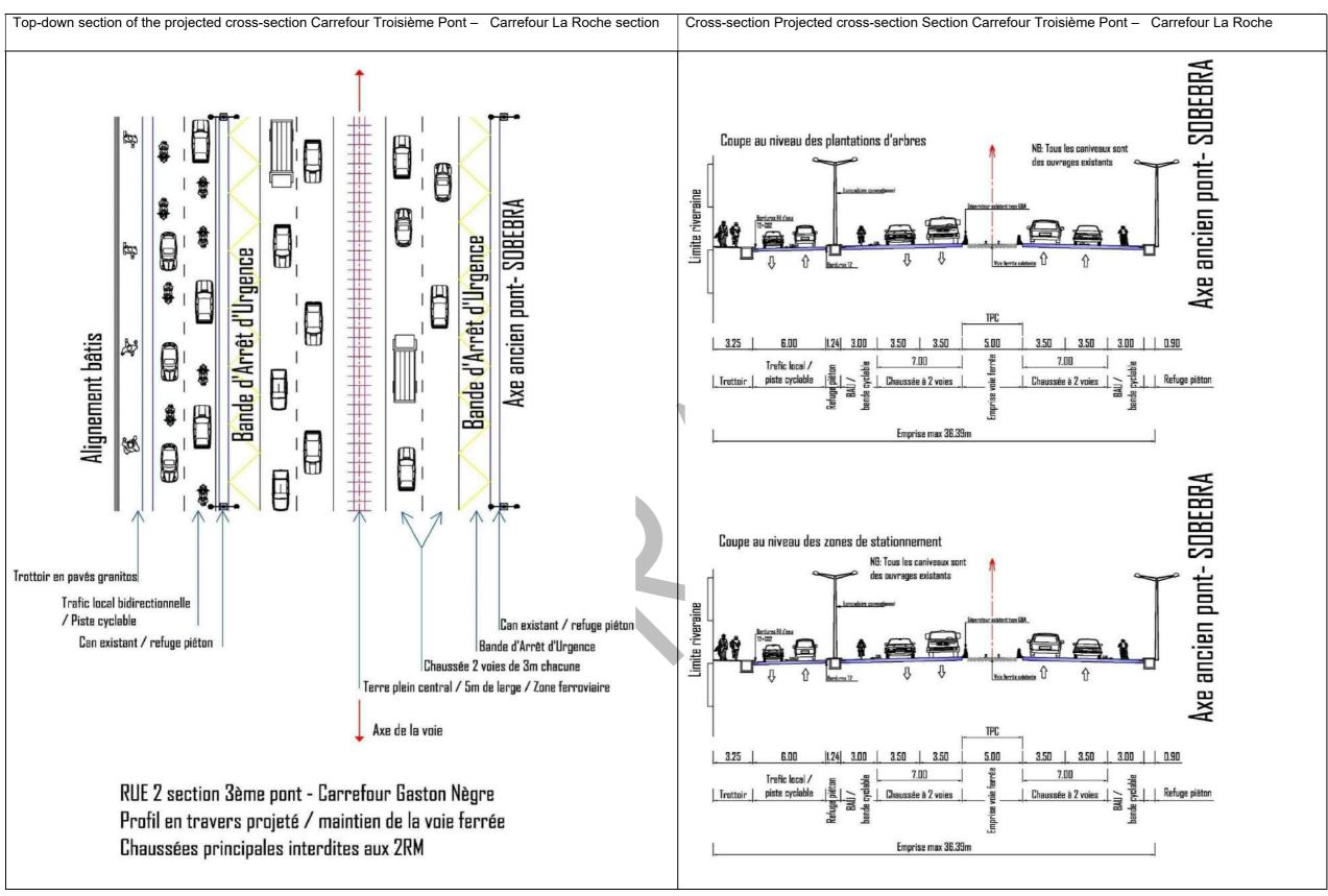
Figure 48: Cross section for the section "Carrefour Troisième Pont – Carrefour La Roche" Source: CECO BTP technical document, May 2022
