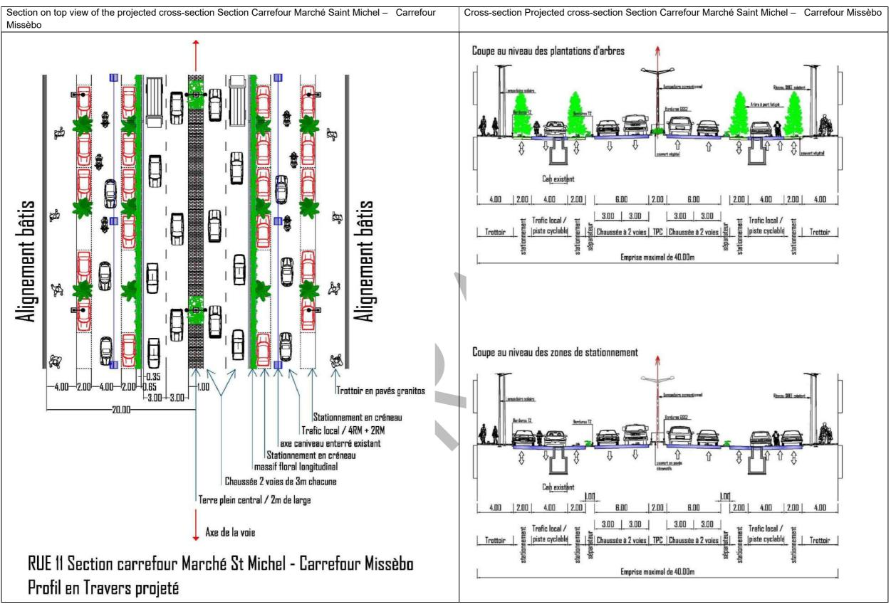
Figure 51: Cross section for the section "Carrefour Marché Saint Michel – Carrefour Missèbo Source: CECO BTP technical document, May 2022
