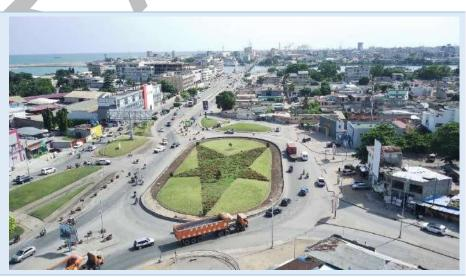
Roundabout of particular shape, solution of visibility problems and large deflections at the level of the branches.
