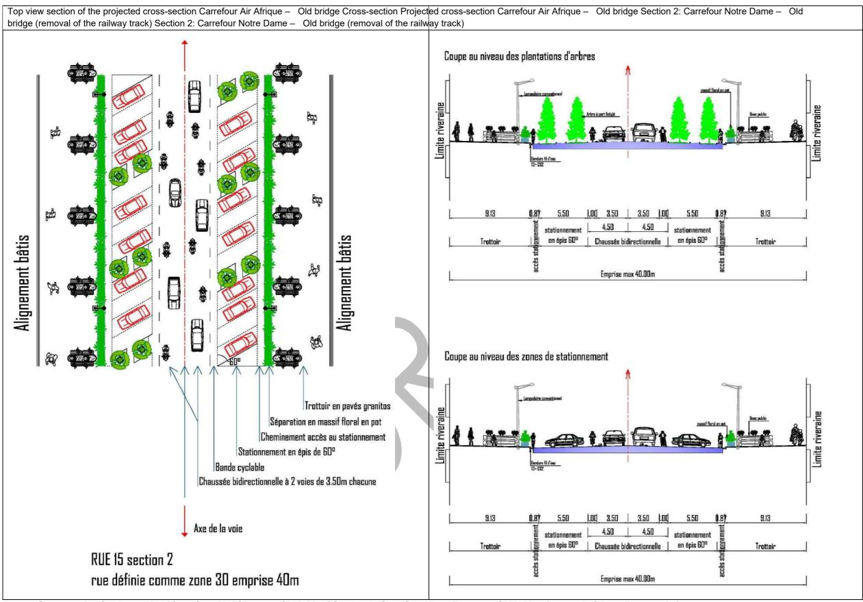
Figure 59: Cross section for the section "Carrefour Air Afrique – Old bridge/ Section 2: Carrefour Notre Dame – Old bridge (removal of the railway tracks) Source: CECO BTP technical document, May 2022
