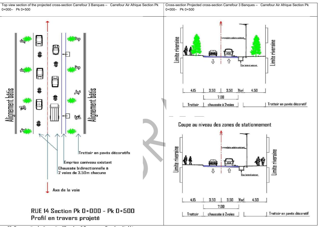
Figure 53: Cross-section for the section "Carrefour 3 Banques – Carrefour Air Afrique Source: CECO BTP technical document, May 2022
