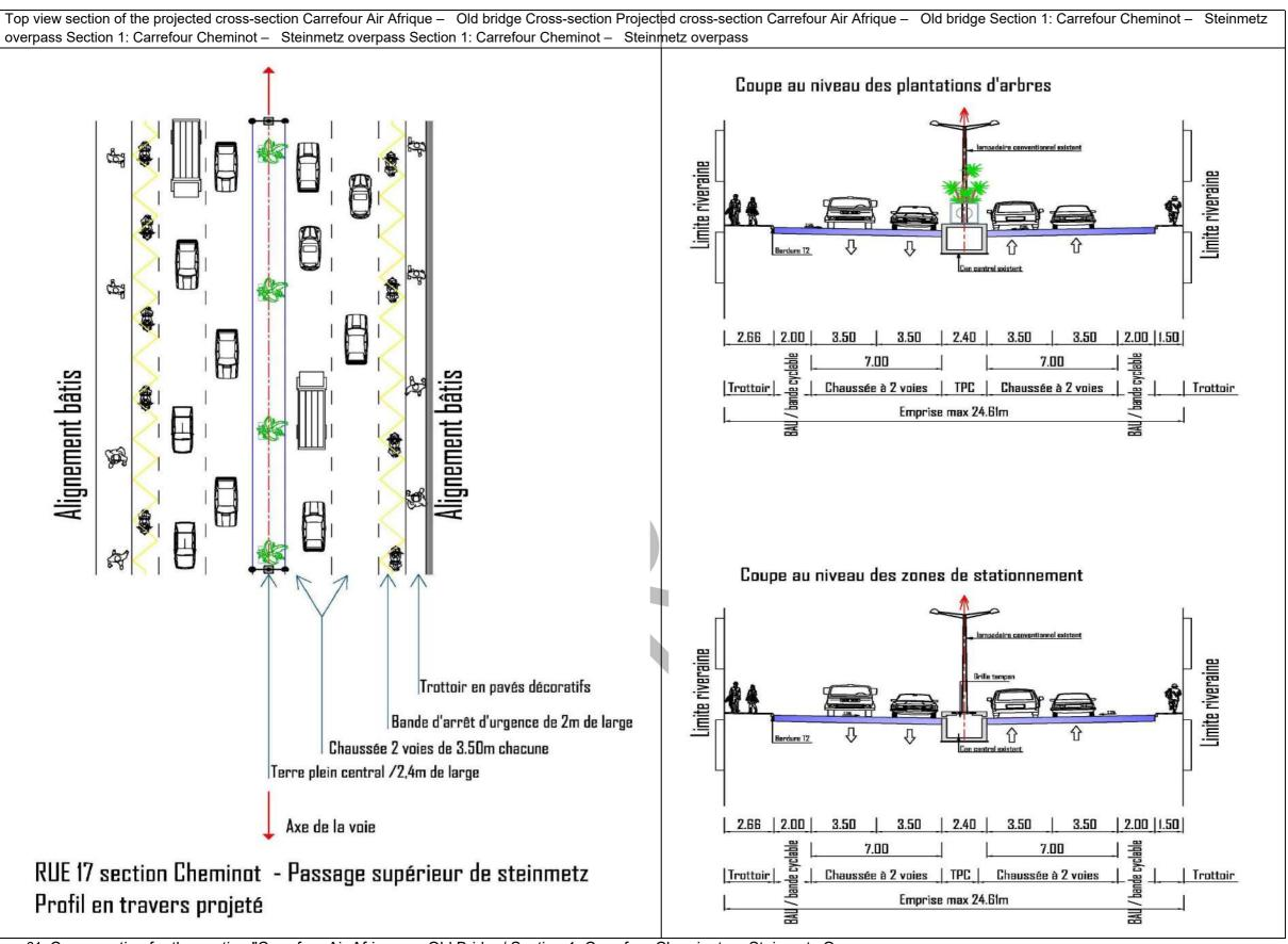
Figure 61: Cross section for the section "Carrefour Air Afrique – Old Bridge/ Section 1: Carrefour Cheminot – Steinmetz Overpass Source: CECO BTP technical document, May 2022
