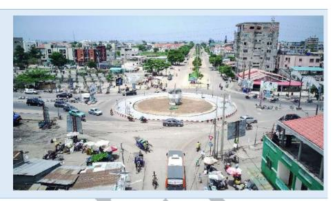
With a roundabout radius of 29m, this intersection is classified as a large roundabout. With a width of 12m for the ring, and an entry and exit lane of 10m; this roundabout in the ring is designed and does not meet CEREMA standards. It is decided to:
