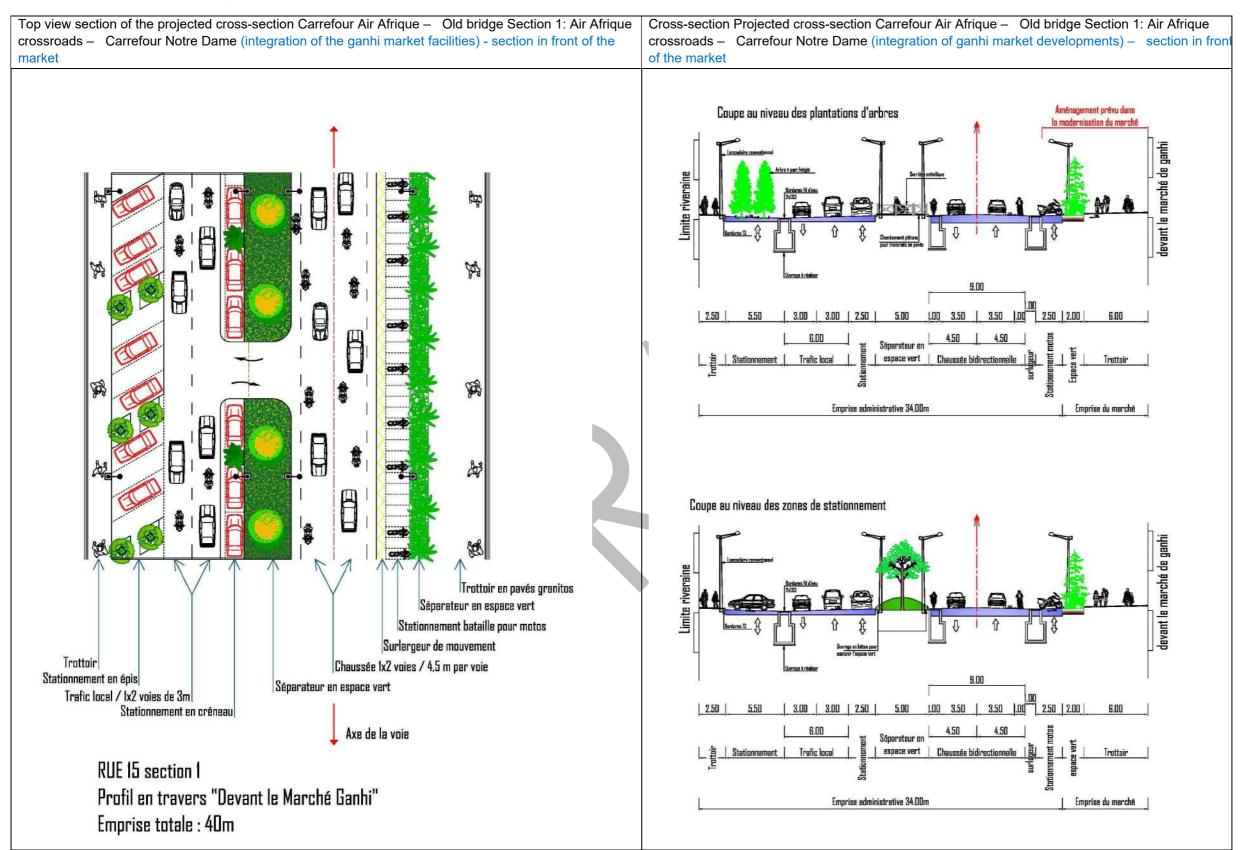
Figure 57: Cross profile for the section "Carrefour Air Afrique – Ancien pont/Section 1: carrefour Air Afrique – Carrefour Notre Dame (integration of the ganhi market developments) – section in front of the market"
