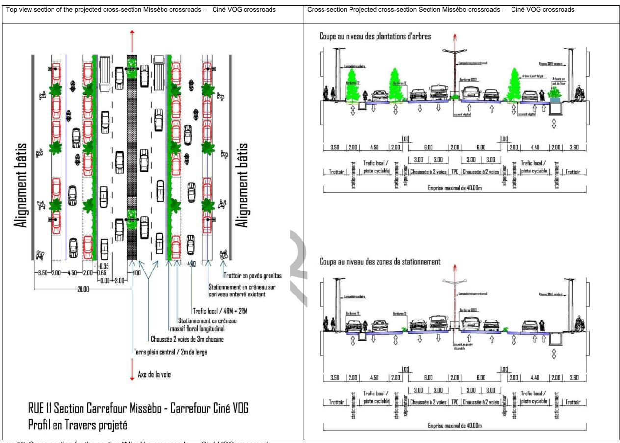
Figure 52: Cross section for the section "Missèbo crossroads – Ciné VOG crossroads Source: CECO BTP technical document, May 2022
