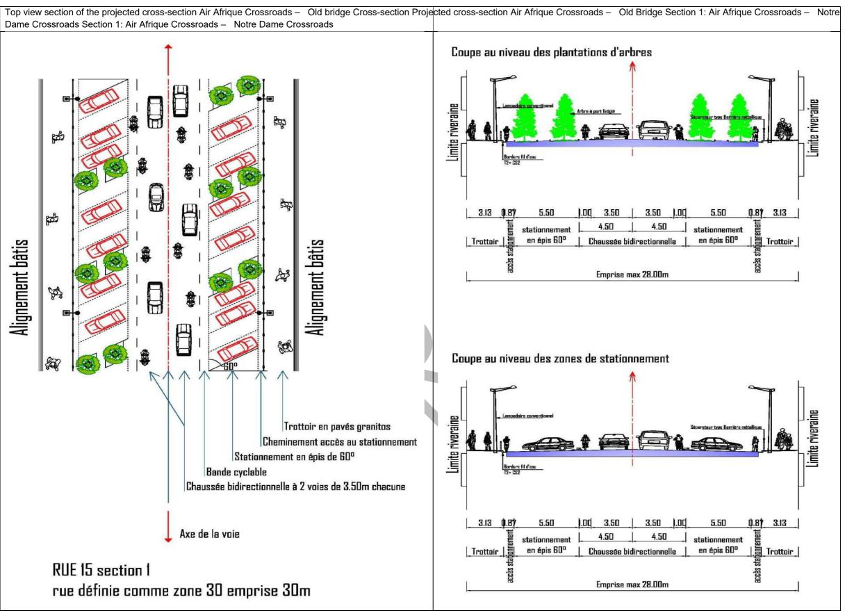
Figure 55: Cross section for the section "Air Afrique Hub – Old Bridge/Section 1: Air Africa Hub – Notre Dame Hub" Source: CECO BTP technical document, May 2022
