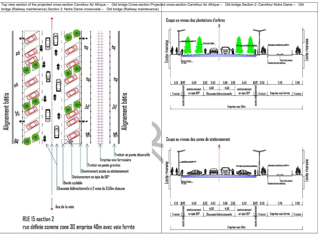
Figure 60: Cross section for the section "Carrefour Air Afrique – Old Bridge/ Section 2: Carrefour Notre Dame – Old Bridge (Maintaining the Tracks)
