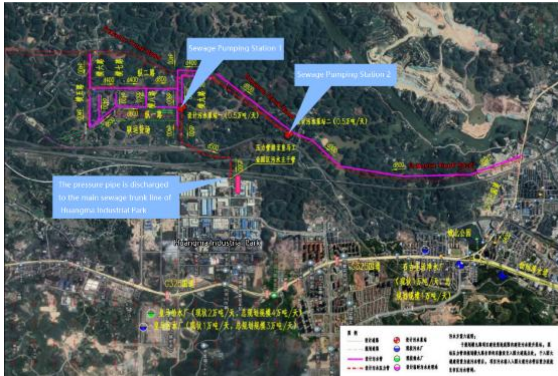
Figure III-18: Sewage Drainage Scheme
